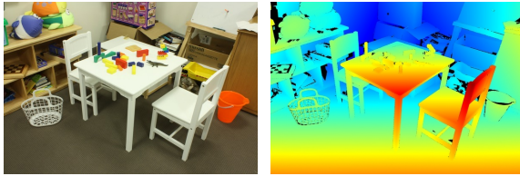
Binocular Stereo, Fig. 5 Middlebury benchmark (an example scene image and its ground truth disparity map).
